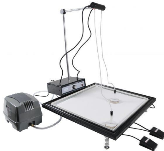
Figure 4.1: Experiment set-up of elastic collision in two dimension.
